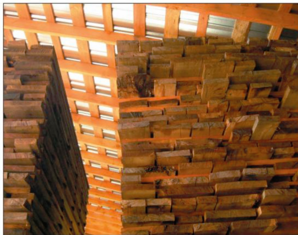
New-sawn oak boards dry for a year in this breezy, shady shelter.
